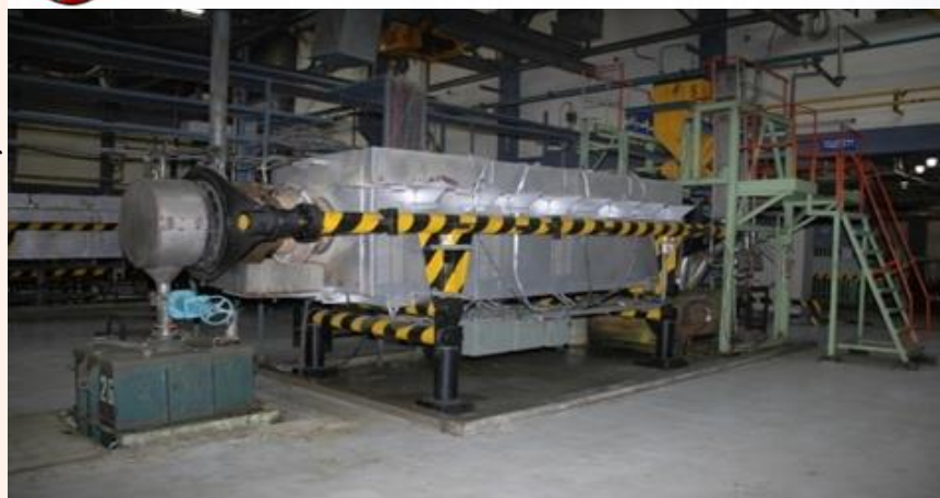
Figure-3: Unique design of baffle cage for rotary furnaces and the picture of calcination furnace
