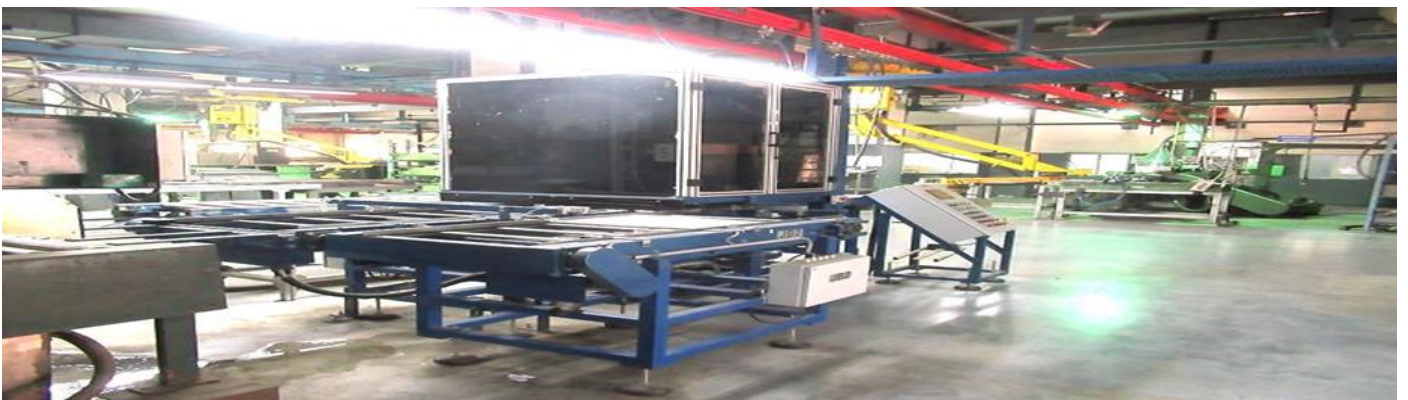
Figure-6: Automatic pellet stacking machine
