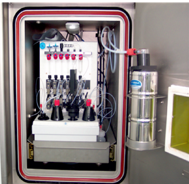
Lead shielded Hot-cells (left) where the PET-radioisotopes produced in the cyclotron are converted to PET-Radiopharmaceuticals. Centre - Automated 18F-FDG synthesis module housed in hot-cell. Right - Dispensing module housed in a hot-cell to aseptically dispense 18F-FDG for transport to PET-imaging centres.
