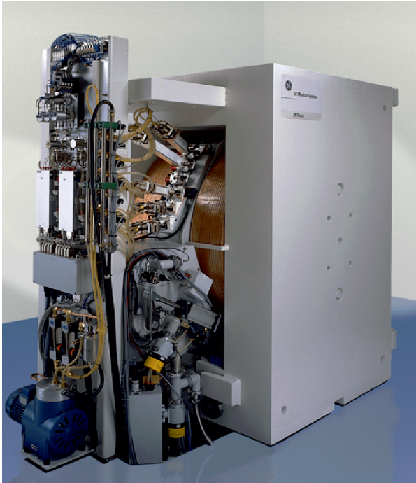
Medical Cyclotron (left) and targets (right) where the PET radioisotopes are produced
