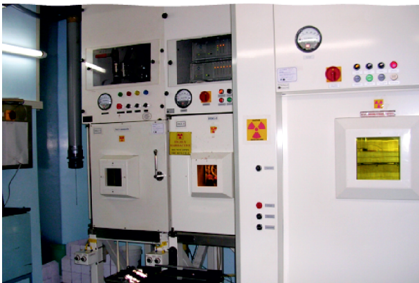
Medical Cyclotron (left) and targets (right) where the PET radioisotopes are produced
